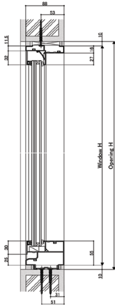
< Vertical section: Single fixed window (IG unit) >
